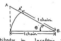
It is the correction to be applied in the field at every chain length and every point, where the slope changes
